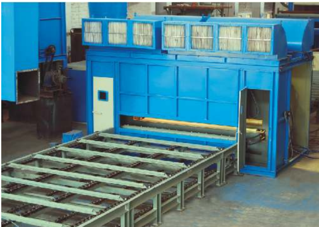
Paint Spray Booth with X Manipulator & Slat Conveyor System
