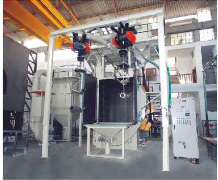
MECSHOT Airless 'Y' Hanger Type Shot Blasting M/c with Motorized Trolley
