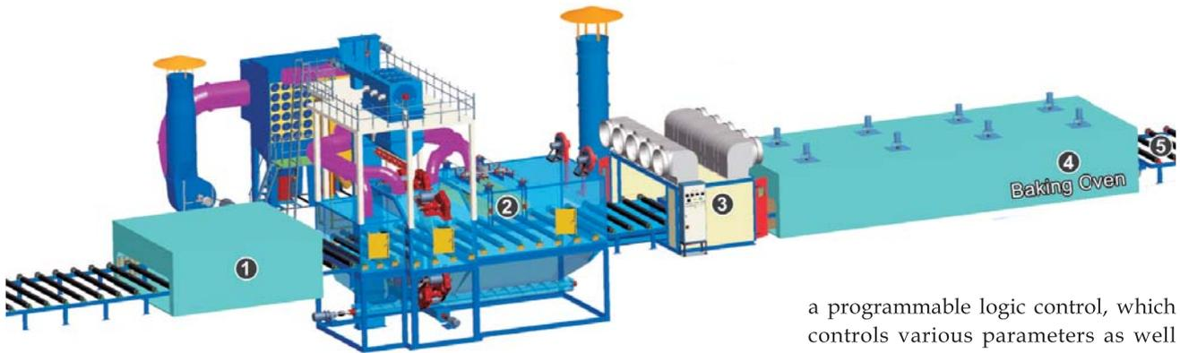
the media recovery hopper, conveyed by screw conveyors to the boot of the bucket elevator. In the separator drum the media gets air washed and separated into over & under sized media. The usable media is finally transferred to the storage tank for reuse. The blast wheels are dynamically balanced. The maintenance of the wheels can be easily carried out by simply replacing normal wearing parts like blades and liner plates.
